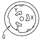
VIEW-B (CONNECTOR FACE VIEW CS8365C PLUG-ENLARGED)
